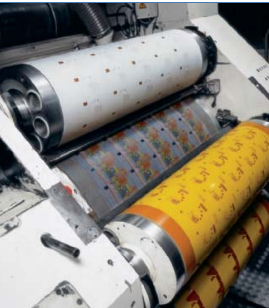
Plate cylinders for printing €50 banknotes and a rubber printing blanket in an offset printing machine.
