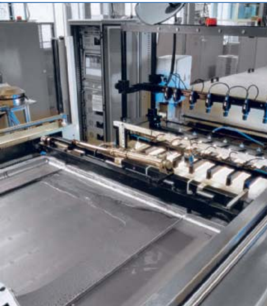
A silkscreen printing machine for applying colour-shifting ink to €50 banknotes.
