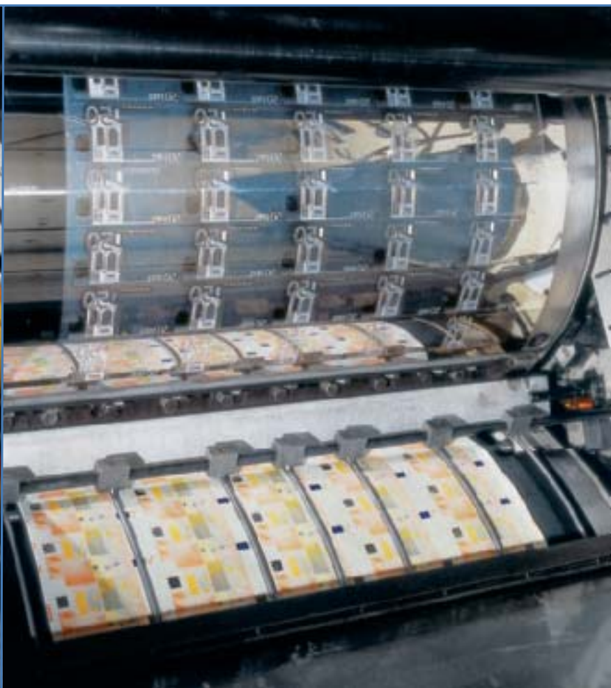
Plate cylinder for printing €50 banknotes in an intaglio printing machine.
