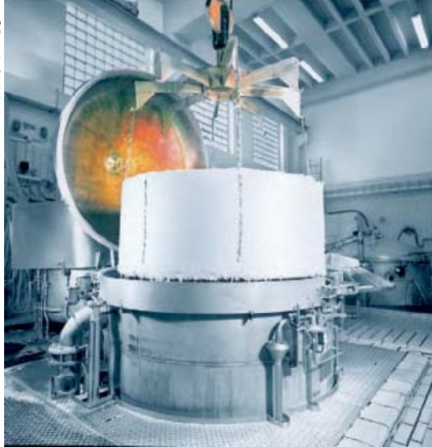
Cotton fibres after the bleaching process.
